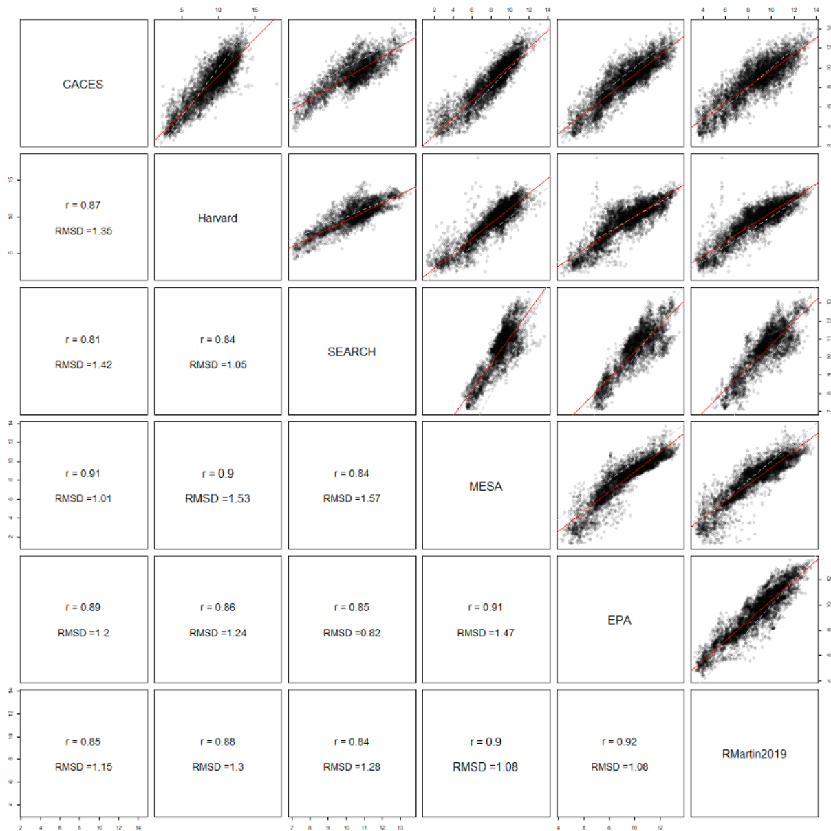
Figure S5: Scatterplot matrix for 2010 rural tract-level PM 2.5 (E-US only). Same as Fig 1, but for rural locations in E-US only. Scatterplots in the upper right show pairwise tract-level predictions from each model. Dashed line shows 1:1 line, red line shows linear trendline. Corresponding boxes in the bottom left show Pearson's correlation ( r ; unitless) and root mean squared difference (RMSD; \mu\text{g}/\text{m}^3 ) between model predictions.
