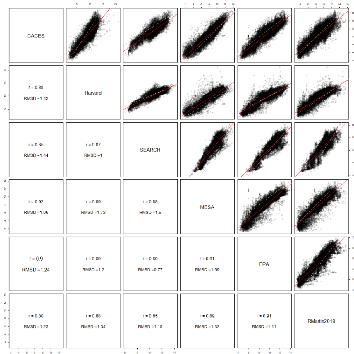
Figure S4: Scatterplot matrix for 2010 rural tract-level PM_{2.5} . Same as Fig 1, but for rural locations only. Scatterplots in the upper right show pairwise tract-level predictions from each model. Dashed line shows 1:1 line, red line shows linear trendline. Corresponding boxes in the bottom left show Pearson's correlation ( r ; unitless) and root mean squared difference (RMSD; \mu g/m^3 ) between model predictions.
