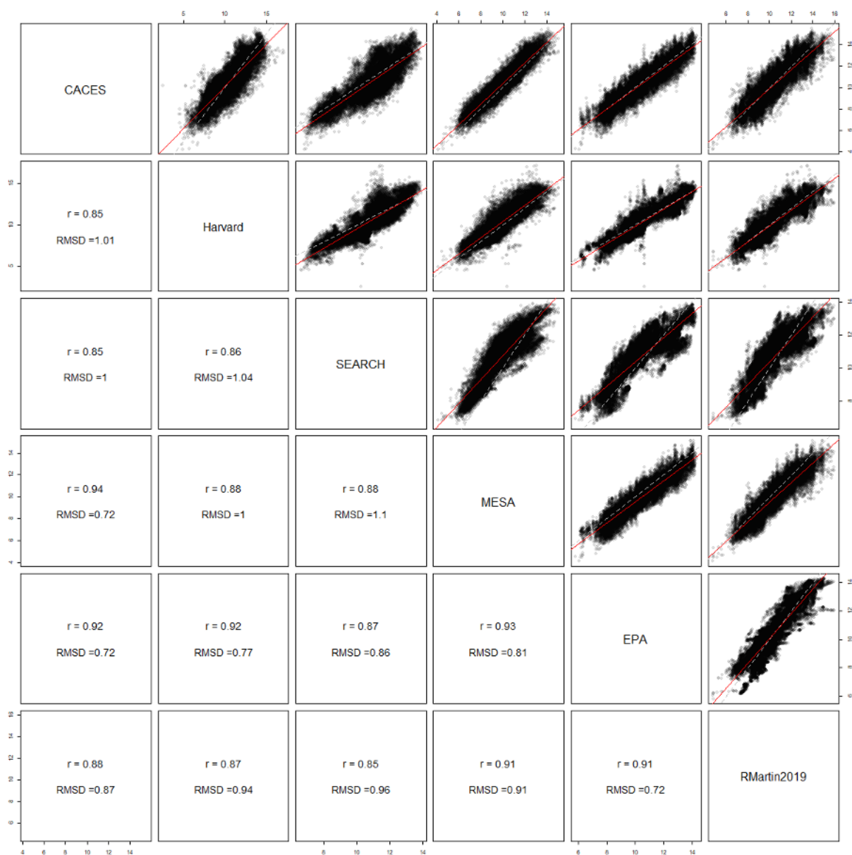
Figure S3: Scatterplot matrix for 2010 urban tract-level PM_{2.5} (E-US only). Same as Fig 1, but for urban locations in E-US only. Scatterplots in the upper right show pairwise tract-level predictions from each model. Dashed line shows 1:1 line, red line shows linear trendline. Corresponding boxes in the bottom left show Pearson's correlation ( r ; unitless) and root mean squared difference (RMSD; \mu g/m^3 ) between model predictions.
