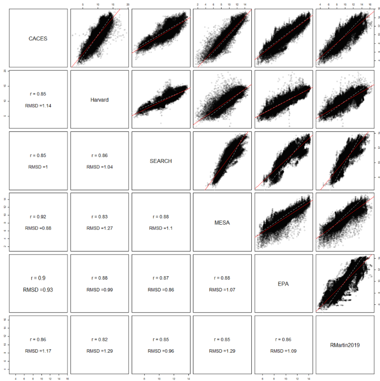
Figure S2: Scatterplot matrix for 2010 urban tract-level PM_{2.5} . Same as Fig 1, but for urban locations only. Scatterplots in the upper right show pairwise tract-level predictions from each model. Dashed line shows 1:1 line, red line shows linear trendline. Corresponding boxes in the bottom left show Pearson's correlation ( r ; unitless) and root mean squared difference (RMSD; \mu g/m^3 ) between model predictions.
