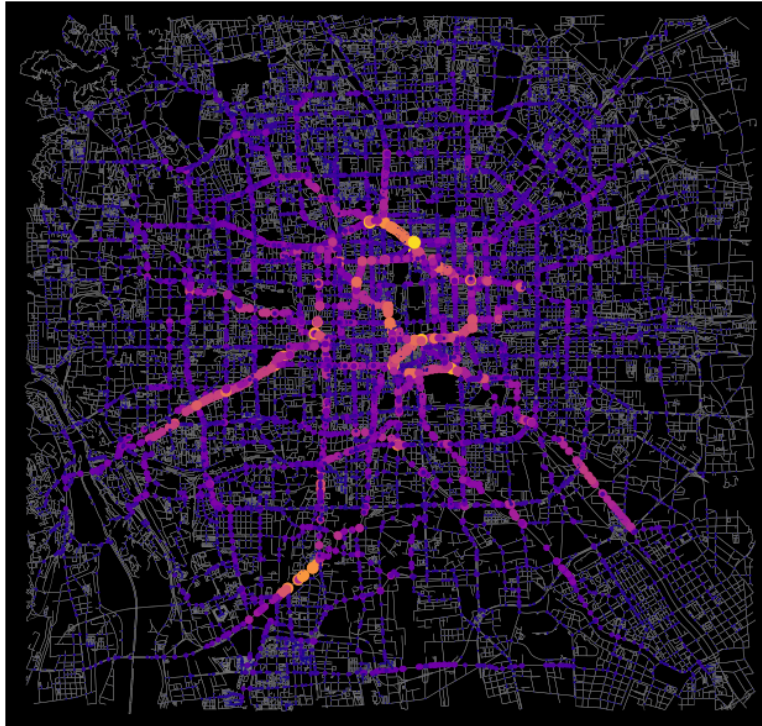
Figure 2. Spatial distribution of node betweenness centrality (weighted by edge length) for Beijing, China (yellow nodes are more central). We observe the emergence of non-trivial patterns of large BC nodes (Data from OSM).
